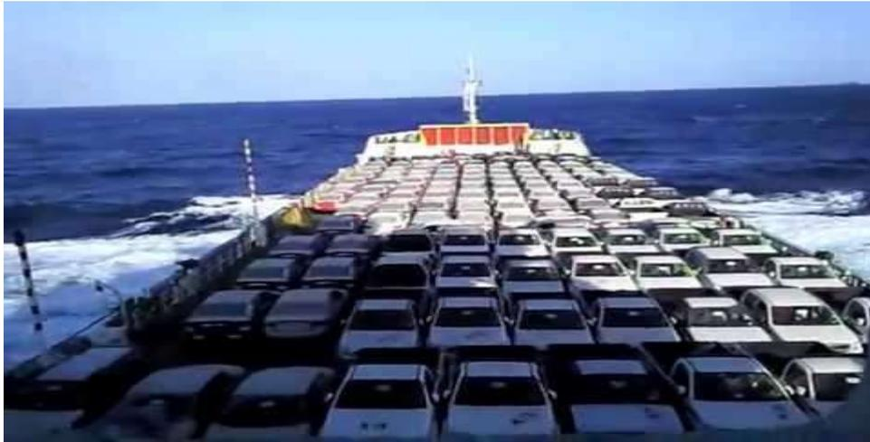
**Breakbulk:** Break bulk cargo are goods that must be loaded individually are not in an intermodal container this sort of cargo is called general cargo ships.
