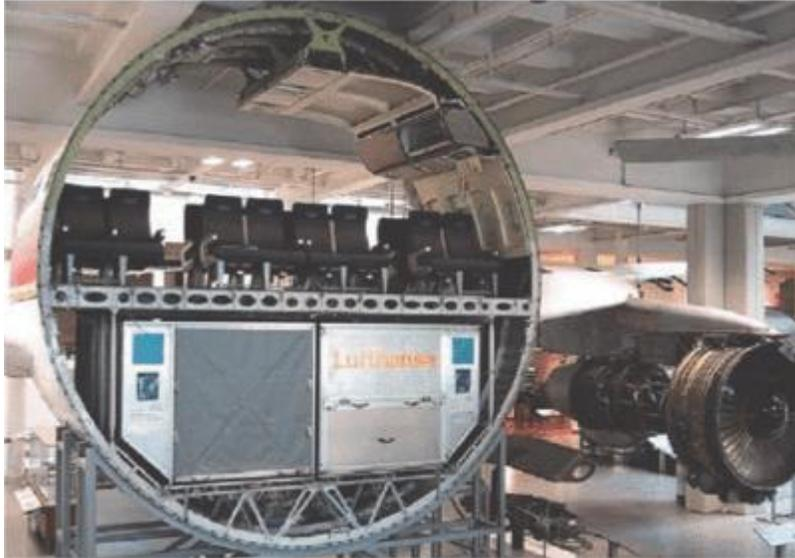
Figure 1.2. Airbus A300 aircraft cross-section displaying cargo containers on lower deck.
